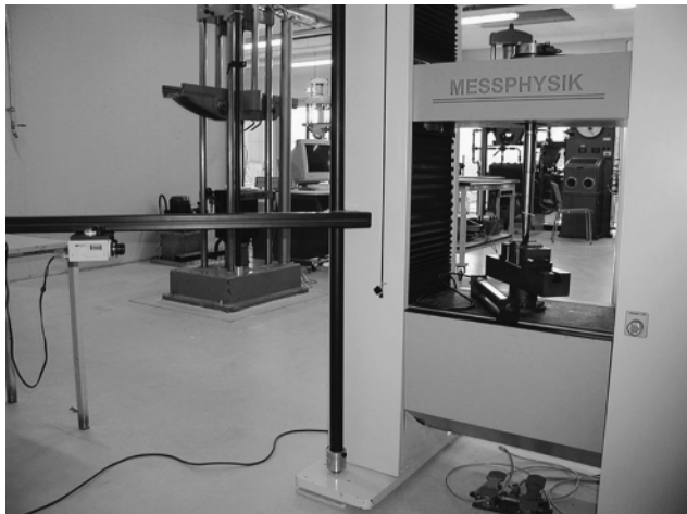
Figure 6 Experimental setup with video extensometer and Shimadzu Autograph.
